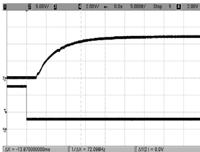
Enable Start-up (Vin=48V, Iout=5A, Cload=1000uF Ta=+25°C) Trace 2=Output, Trace 4= Enable.
